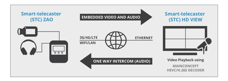
Soliton Systems has licensed MainConcept's HEVC/H.265 Decoder SDK to meet their requirements of multi-stream real-time decoding on standard computer hardware in their STC HD View software. These four streams can further feed into the editor's broadcast system via HD-SDI. Moreover, the STC HD View application can archive incoming streams to local files for long-time storage and later playback.
